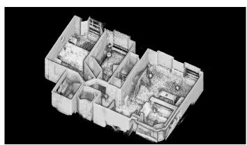
Capture and create real estate and commercial property floorplans with informative 360° panoramic photography for enhanced property surveys. 3D measurable information and imagery captured with the ZEB PANO uses the leading SLAM algorithm to automatically and accurately position panoramic photos and enables the creation of both 2D and 3D property floorplans.
